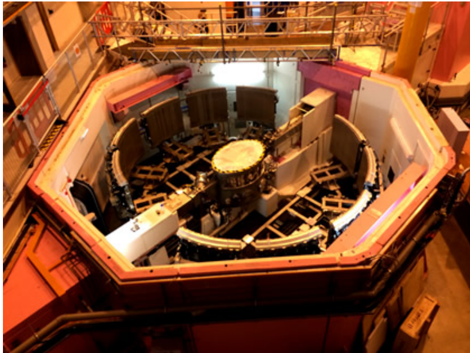
ISIS TS2 instrument WISH sample environment and detector array, exposed for renovation.
